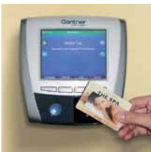
GAT locking system with central information display: The compartment is opened by data carrier directly on the locker, whereas the central display provides information about which compartments are in use and which compartments are free.
