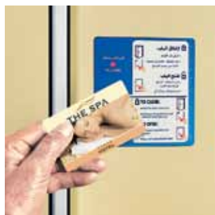
GAT locking system with central information display: The compartment is opened by data carrier directly on the locker, whereas the central display provides information about which compartments are in use and which compartments are free.
