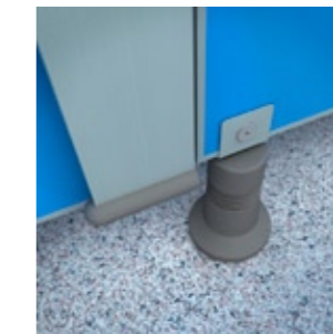
Adjustable foot with screw calibrator hidden by bellows type sleeve. Made from grey glass filled nylon it also acts as the hinge pivot.
