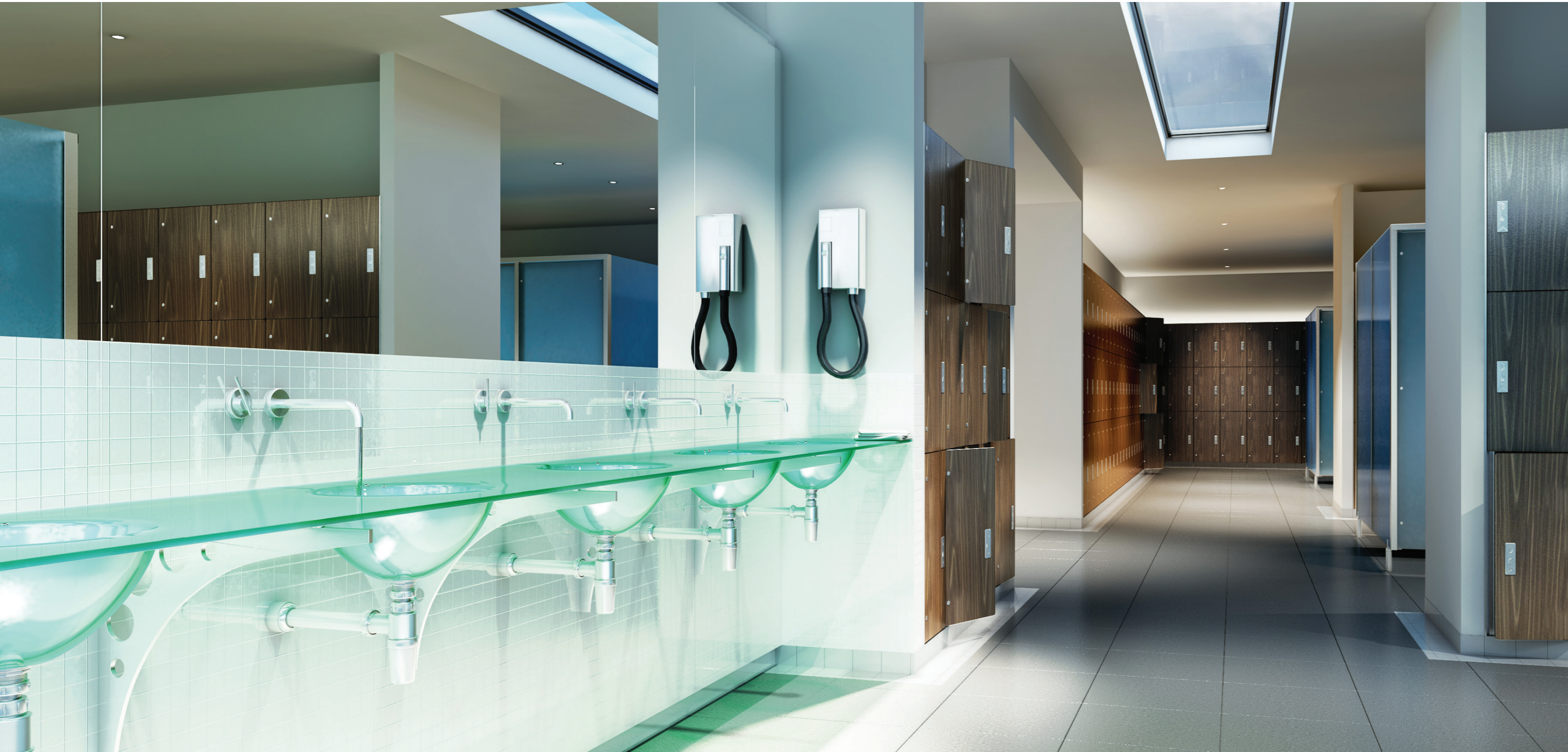
slab vanities in prefabricated 19mm glass. fusion lockers right and left hung, in wood veneer.
