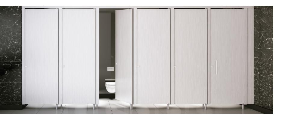
Features: Visible full aluminium frame. Available up to 2500mm with 100mm floor gap. Also available in standard height of 2000mm with 150mm floor gap. Finished door thickness of 27mm. Anti-fingertrap feature. Concealed self-closing door closer in foot. Pivoted door. Aluminium fittings. Machined aluminium lock locates into post. Core sourced from legal and sustainable sources. Can be supplied to meet NAUF criteria. Emergency release. 10 year warranty. Also available in:
