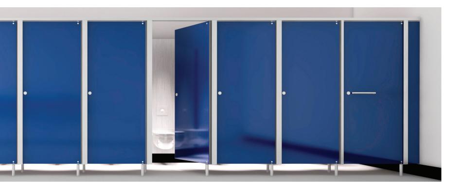
Features: Visible full aluminium frame. Standard height of 2000mm with 150mm floor gap. Available in full height version up to 2500mm with 100mm floor gap (as Icon Glass Tall). Finished door thickness is either 10mm back painted glass or 10.76mm laminated glass. Anti-fingertrap feature. Concealed self-closing door closer in foot. Pivoted door. Aluminium fittings. Machined aluminium lock locates into post. Glass can match any RAL colour. Emergency release. 10 year warranty.
